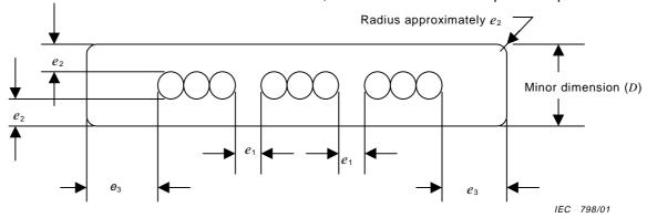
NOTE This figure is to illustrate the thickness of sheath and clearance referred to in table 5 and does not represent an actual design.
